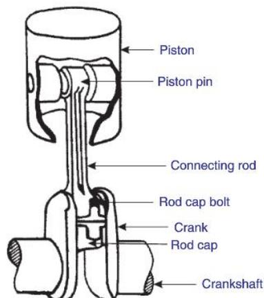
**Crank, Crank Shaft & Crank Case:**
