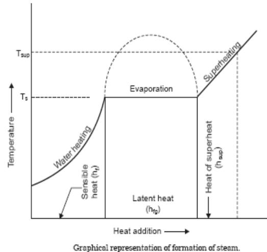
Again, if supply of heat to the dry and saturated steam is continued at constant pressure there will be increase in temperature and volume of steam. The steam so obtained is called *superheated steam* and *behaves like a perfect gas*.
