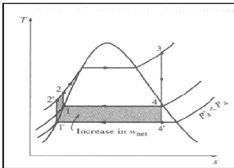
Lowering the operating pressure of the condenser lowers the temperature at which heat is rejected. The overall effect of lowering the condenser pressure is an increase in the thermal efficiency of the cycle.
