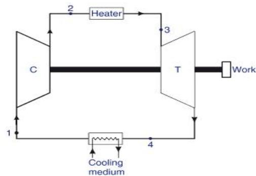
$$\eta_{\text{air-standard}} = \frac{\text{Work done}}{\text{Heat received}} = \frac{\text{Heat received/cycle} - \text{Heat rejected/cycle}}{\text{Heat received/cycle}}$$
