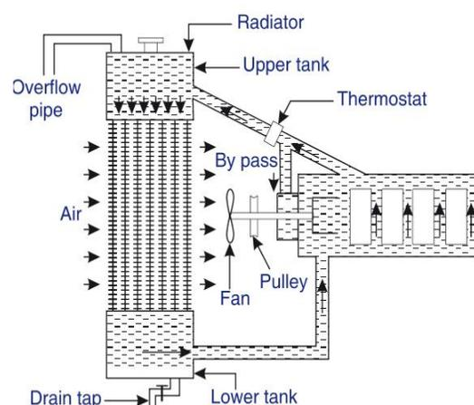
Thermostatically controlled cooling system.
