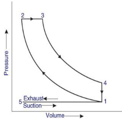
Theoretical *p-V* diagram of a four-stroke Diesel cycle.
