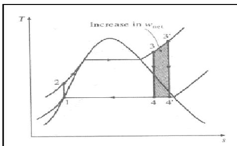
The average temperature at which heat is added to the steam can be increased without increasing the boiler pressure by superheating the steam to high temperatures.
