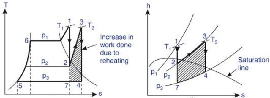
The steam as at state point 1 (i.e., pressure  $p_1$  and temperature  $T_1$ ) enters the turbine and expands isentropically to a certain pressure  $p_2$  and temperature  $T_2$ . From this state point 2 the whole of steam is drawn out of the turbine and is reheated in a reheater to a temperature  $T_3$ . This reheated steam is then readmitted to the turbine where it is expanded to condenser pressure isentropically
