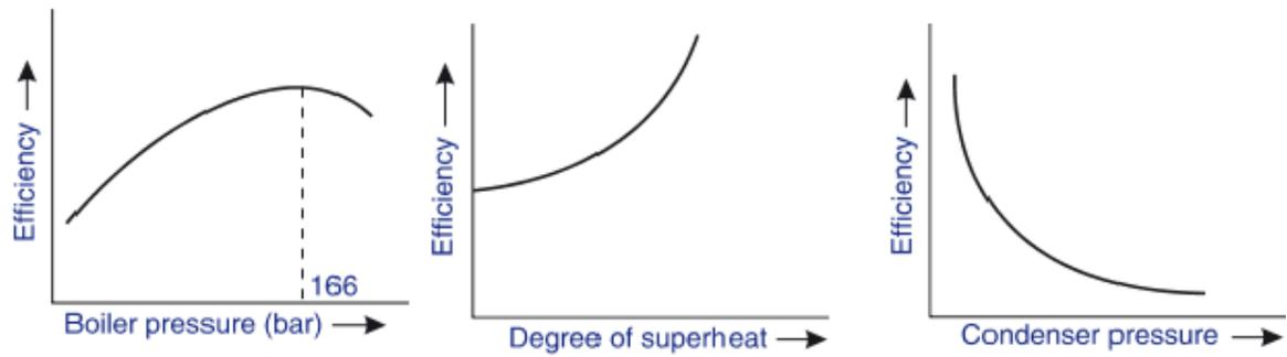
The thermal efficiency of the Rankine cycle is also *improved* by the following methods :
