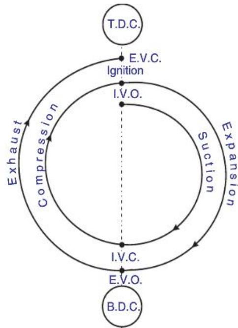
. Theoretical valve timing diagram (four-stroke Otto cycle engine).
