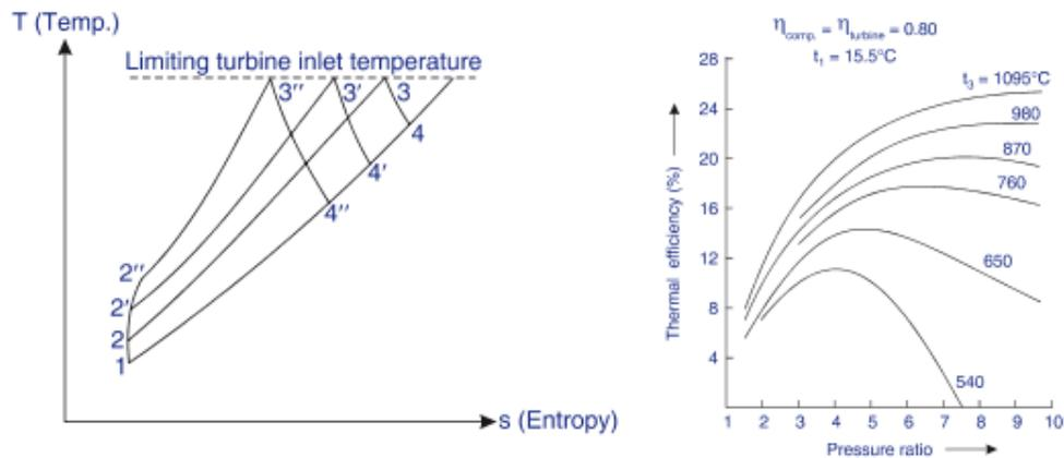
As the pressure ratio increases, the thermal efficiency also increases until it becomes maximum and then it drops off with a further increase in pressure ratio. Further, as the turbine inlet temperature increases, the peaks of the curves flatten out giving a greater range of ratios of pressure optimum efficiency.
