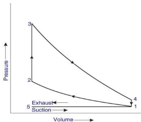
Theoretical p-V diagram of a four-stroke Otto cycle engine.
