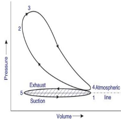
Actual *p-V* diagram of four-stroke Diesel cycle.
