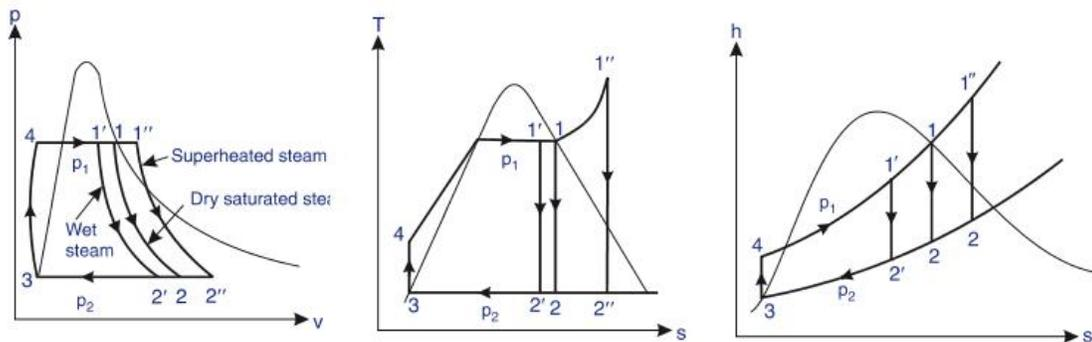
The steam leaving the boiler may be dry and saturated, wet or superheated. The corresponding T-s diagrams are 1-2-3-4-1; 1-2-3'-4'-1 or 1-2-3''-4''-1
