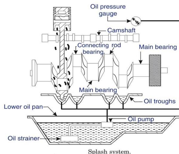
into holes of big end bearing .Due to splash of oil it reaches the lower portion of cylinder wall crankshaft and other parts requiring lubrication. Surplus oil eventually flow to oil sump
