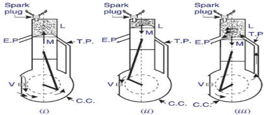
L = Cylinder, E.P. = Exhaust port, T.P. = Transfer port, V = Valve, C.C = Crank chamber
