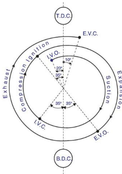
. Actual valve timing diagram (four-stroke Otto cycle engines).
